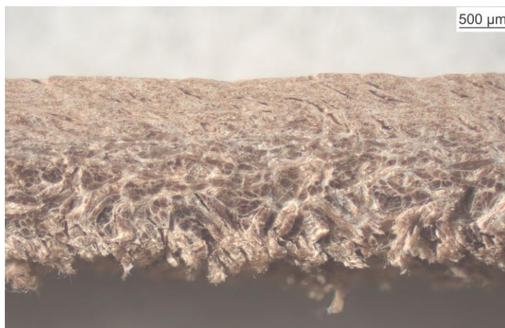
On the photo: bovine, full grain crust with its more dense, horizontal fiber structure on the grain side, and the more open, longer and vertical fibers towards the flesh side. Photo courtesy of Filk Freiberg Institute gGmbH , 2026
