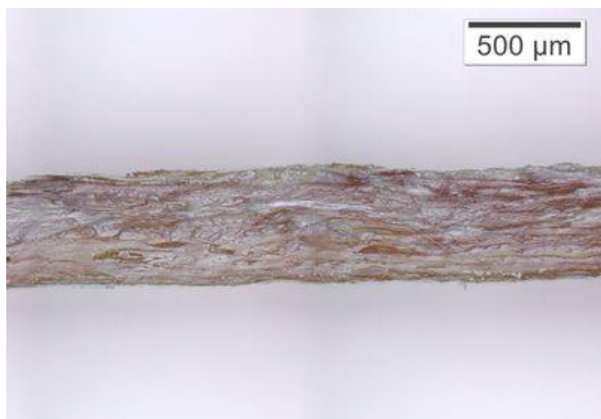
On the photo: parchment from bovine split. A rigid material because fibers are “glued” together after drying. Photo courtesy of Filk Freiberg Institute gGmbH , 2026
