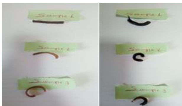
Figure 6. Unhaired and hair-on leather samples after shrinkage test, respectively
