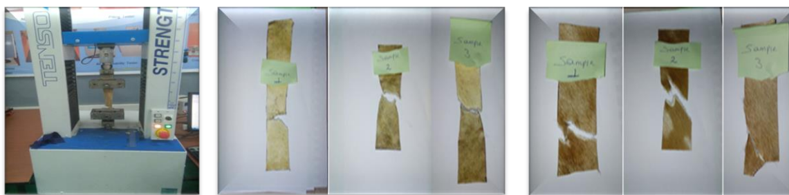
Figure 2. Measuring tensile strength (left); samples from unhaired traditional cowhide leather (center); samples from hair-on traditional cowhide leather (right)
