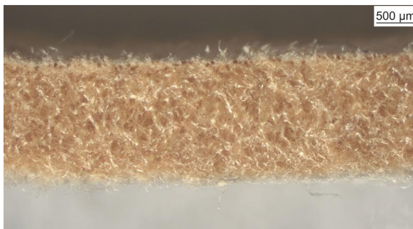
On the photo: chamois tanning leather: the grain has been removed, the remaining reticular layer of the hide shows excellent fiber separation which results in a very soft and plyable article. Long, thin fibers sticking out of the material. Photo courtesy of Filk Freiberg gGmbH , 2026
