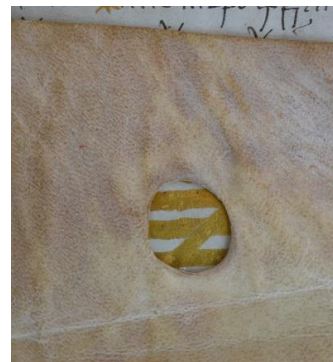
Figure 3. Manufacturing defects specific to parchment: calcium carbonate deposits in hair follicles orifices, and hole formed during drying under tension
