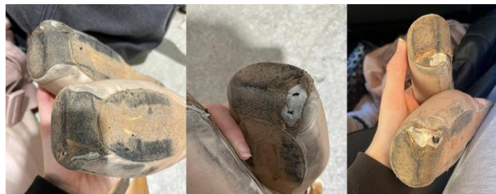
Figure 10. Breakage after 61 hours, breakage after 100 hours and breakage after 145 hours
