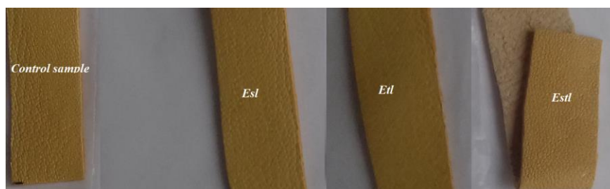
Figure 6. Image of the leathers processed with three structured emulsions: Es, Et, Est, and a control sample
