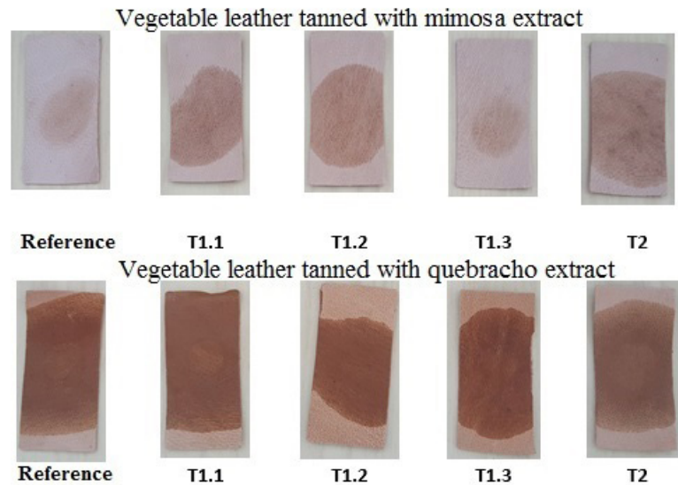
Figure 2. Leather samples during hydrophobisation degree determination
