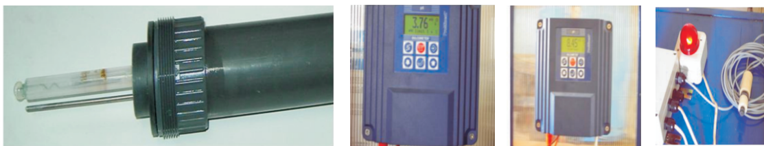
Figure 2. Probe for measuring industrial pH, measurement and pH correction plant and industrial sensor
