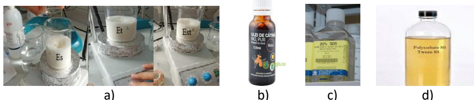
Figure 2. Image of new structured emulsions: a) Es – sea buckthorn oil/sodium dodecyl sulfate/water; Et – sea buckthorn oil/Tween® 80/water; Est – sea buckthorn oil/sodium dodecyl sulfate and Tween® 80 (ratio 1:1)/water; b) sea buckthorn oil; c) sodium dodecyl sulfate; d) Tween 80
