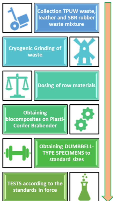
Figure 1. The stages of obtaining polymer biocomposites based on TPU/recycled TPUW/elastomer and protein waste in mixture/PE-g-MA
