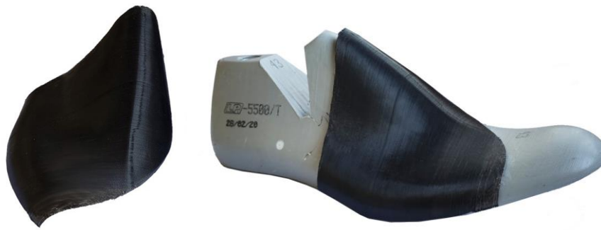
Figure 8. a) The custom insole for the shoe was manufactured using 3D printing; b) The printed insole is attached to the shoe last
