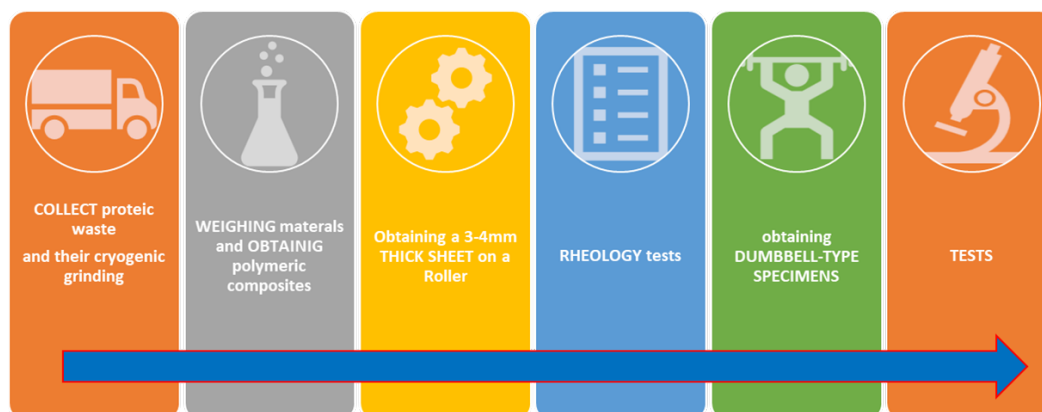
Figure 1. Stages of obtaining polymer composites based on NBR elastomer (butadiene-co-acrylonitrile rubber) and protein waste (PRW)
