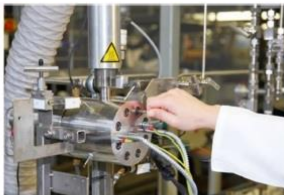
Figure 1. Experimental set-up – high-pressure view-cell for SFE operations
