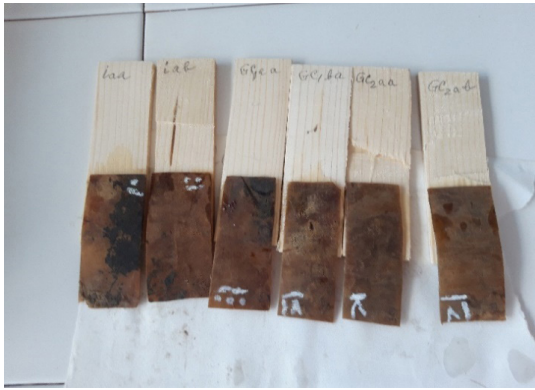
Image 11. Gluing wood and historical parchment hydrated for 72 h in hydroalcoholic solution
