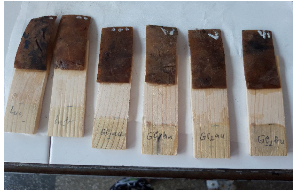
Image 12. Gluing wood and historical parchment hydrated for 72 h in urea solution
