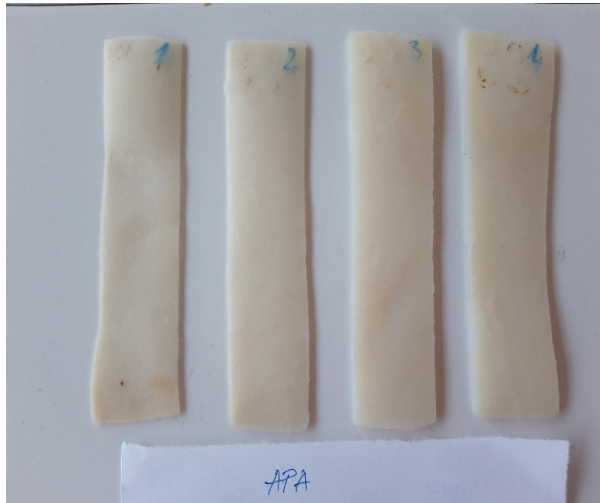
Image 9. New parchment rehydrated in water, after 72 h
