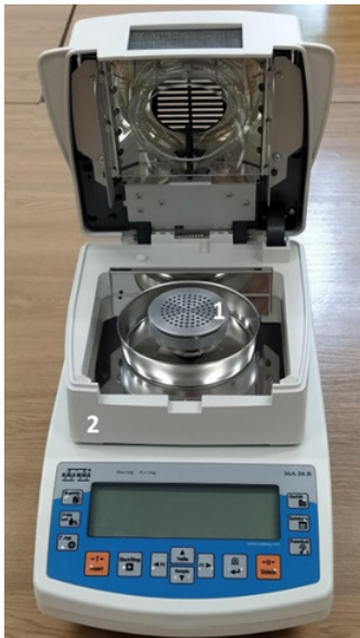
Figure 1. Water vapour permeability testing set for tanned leather: 1 – sampler, 2 – moisture analyser
