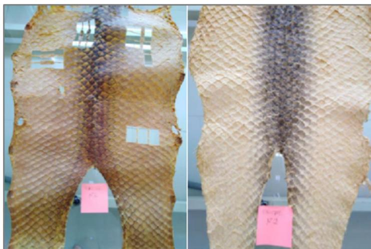
Figure 4. Samples of skins corresponding to tanning processes A and D respectively
