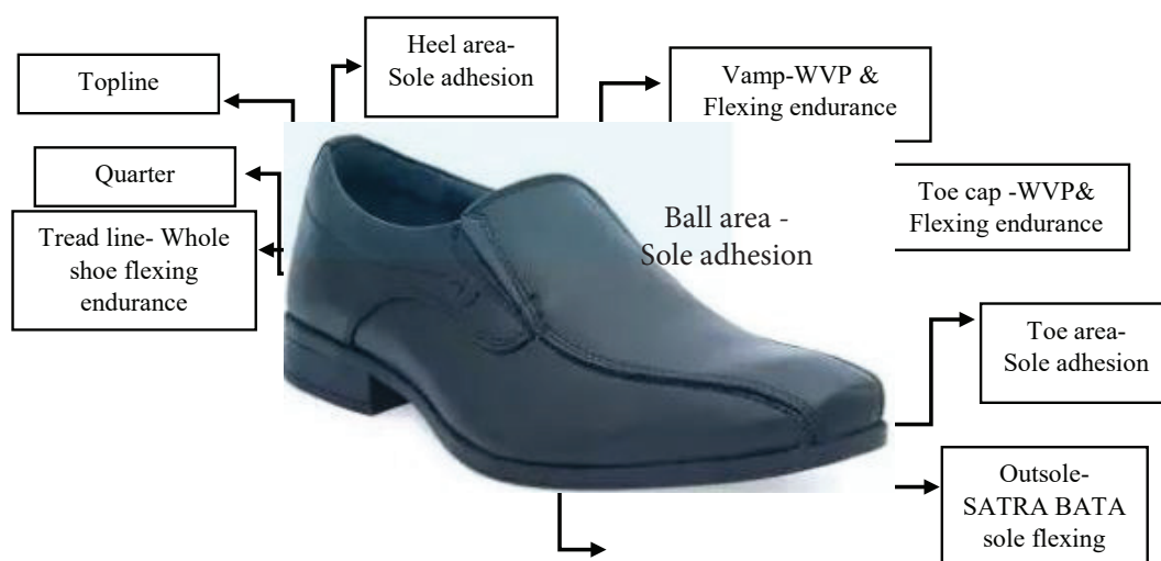
Figure 1. Different parts of a casual shoe with major physical tested sample area
