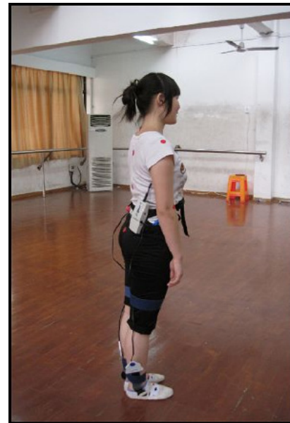
Figure 2. The test situation of the student with insole pressure test device
