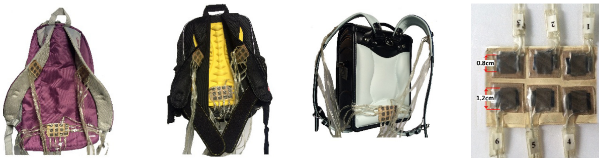
Figure 1. (a) Sensor position distribution backpack A, (b) Sensor position distribution backpack B, (c) Sensor position distribution backpack C, (d) Sensor size
