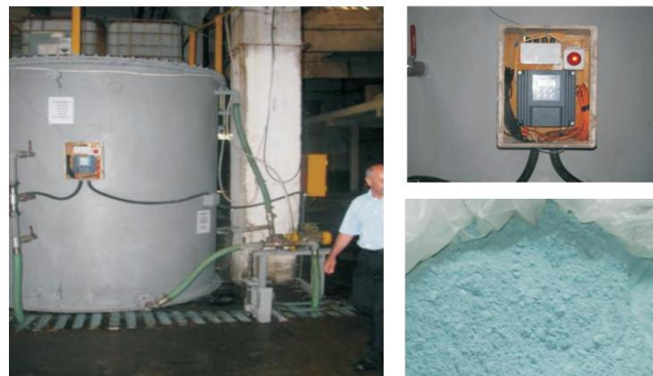
Figure 3. Industrial plant (12,000-14,000 litre tank) for treatment of wastewaters from leather tanning
