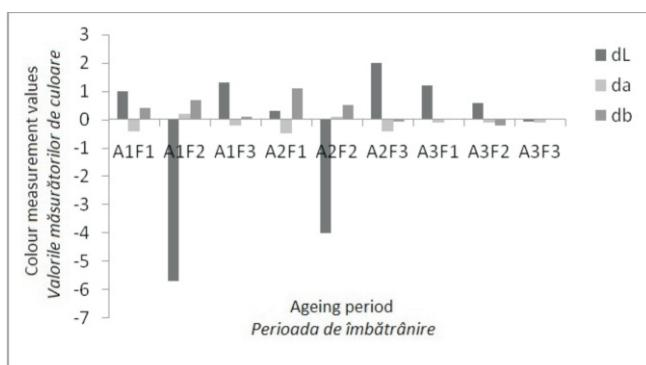
Figure 3. Colour difference values of metal complex dye (1:1) for full chrome suede leather on ageing
