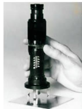
Figure 2. Optical Micrometer
