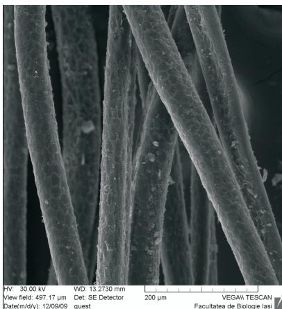
**Figure 3.** Fur hair treated with anionic antistatization mixture (experimental variant  $P_2$ )
