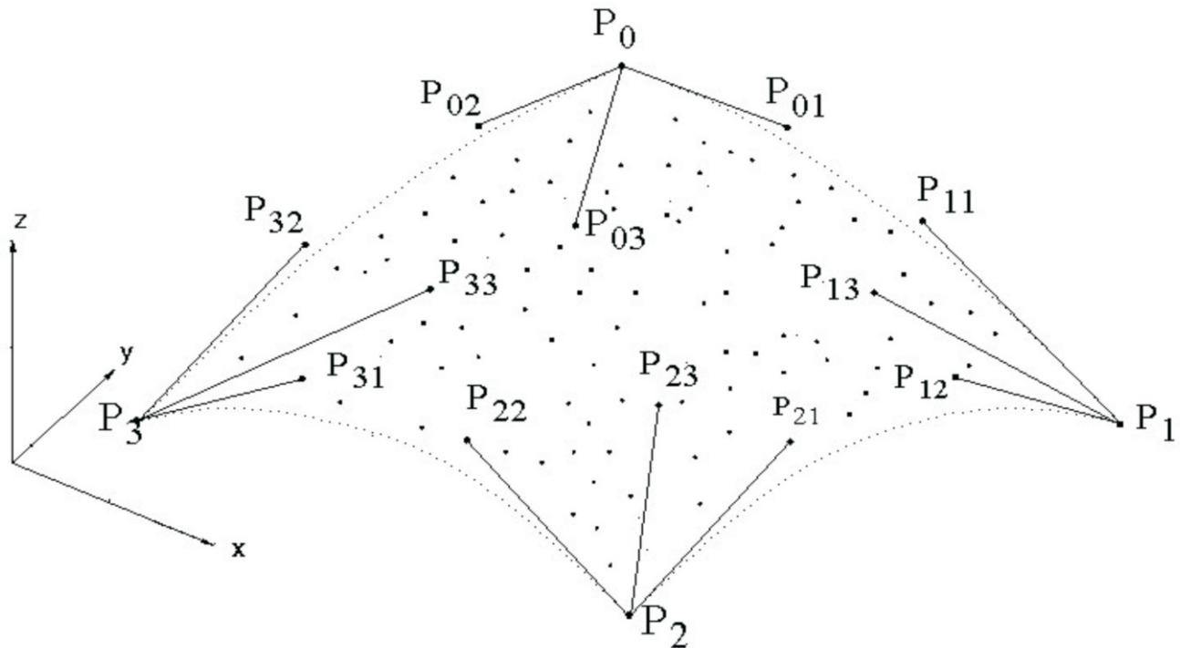
Figure 4. The position of the knots and of the control points for creating a Bézier bi-cubic surface
