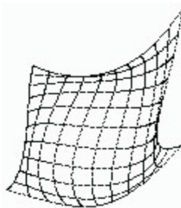
Figure 6. A point on each tangent, together with the 4 knots, determines a Bézier bi-cubic surface
