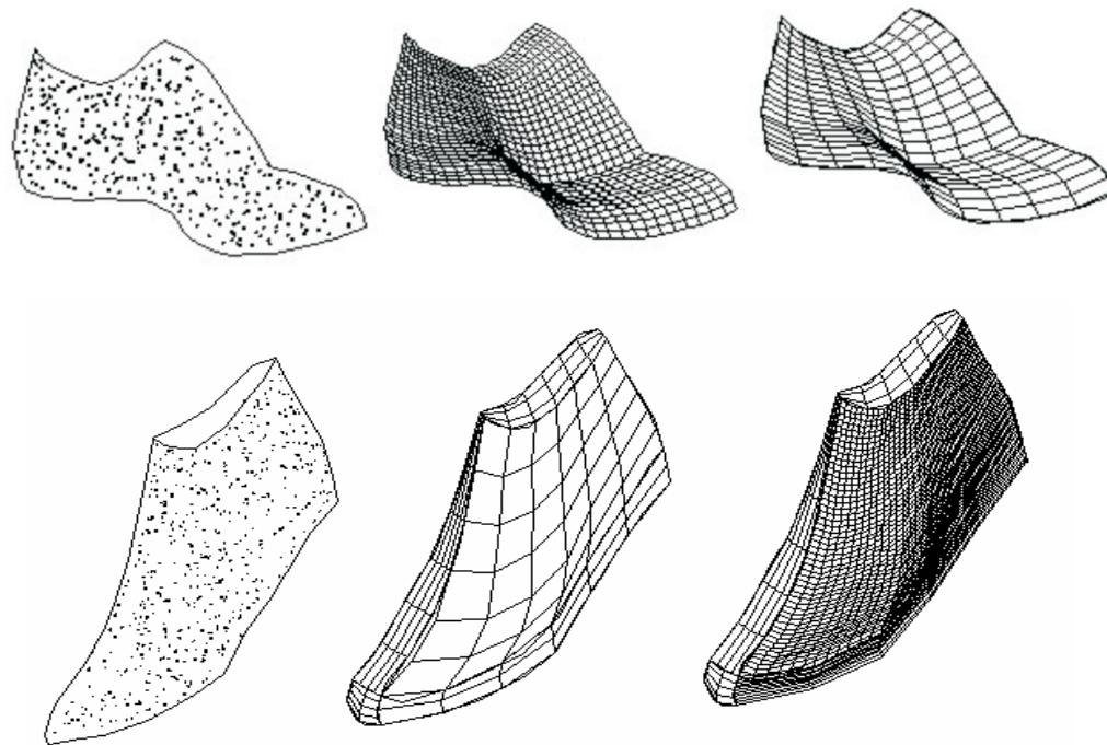
Figure 7. Approximating the set of points of the shoe last with a Bézier bi-cubic surface
